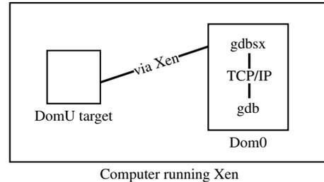
Figure 1: The Xen kernel debugging architecture
