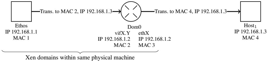
**Figure 3:** Sequence diagram: Ethos sends out a packet
