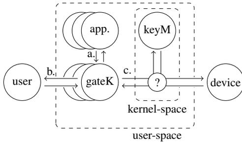
**Figure 2: Ethos’ user-application-gatekeeper-keymaster model**
